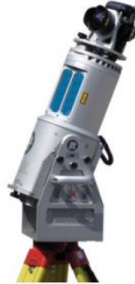
Fig. 5. Laser scanner RIEGL LMS Z420i
