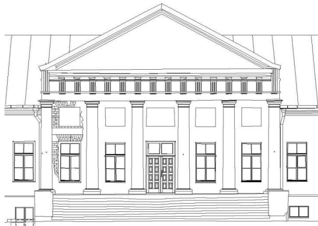
Fig.4. 2D drawing of the central part of the Arnionys mansion-house facade using photogrammetric data
