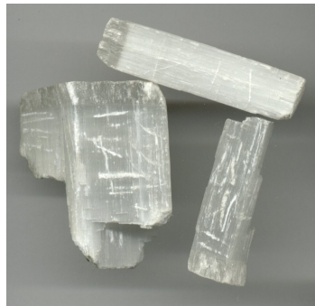
Figure 2. Fibrous gypsum from Brazil (image by Eurico Zimbres FGEL/UERJ).
