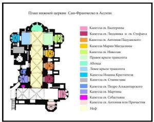
Fig. 4. St. Francis of Assisi Basilica's lower floor plan with chapels at the transept's ends, on right and left sides of the nave and at the nave's west end. 2007 [online 19.06.2017, https://upload.wikimedia.org/wikipedia/commons/a/a5/План\_нижней\_церкви\_Ассизи.jpg]
