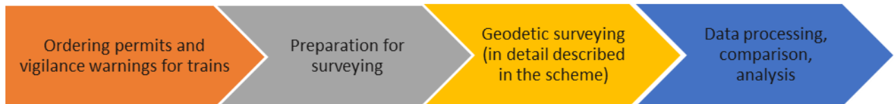
Fig. 1. Technological process of surveying road stretches.
