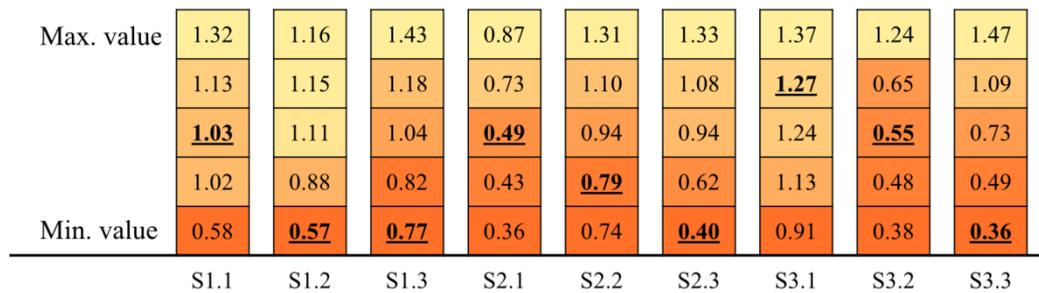
**Figure 5.** Fibre density ratio of longitudinal to transversal directions ( $n_{f,x}/n_{f,yz}$ ) in the range between planes X5 – X9 sorted by the values of the ratio, where bold underlined values represent fibre density ratio in fracture plane
